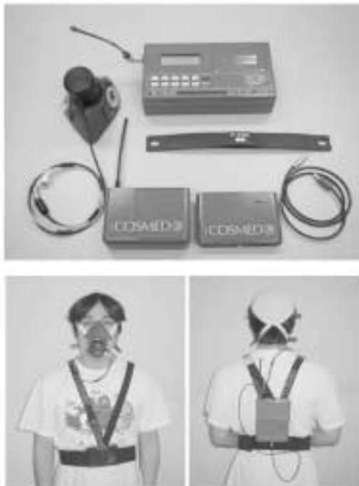
**Fig. 2** A telemetric system used in the present study. The K2 system consists of a face mask, a transmitter, a receiver, an electrode for heart rate recording, a battery, and connectors (top panel). The K2 equipment was worn by a subject (bottom panel). Total carrying mass is 850 g.
